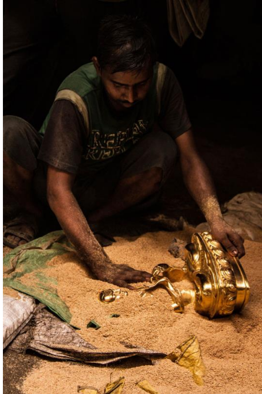
The idols are rubbed in wood husk to give a lustrous effect. Image Source: D'source https://www.dsource.in/resource/brass-work-aligarh
