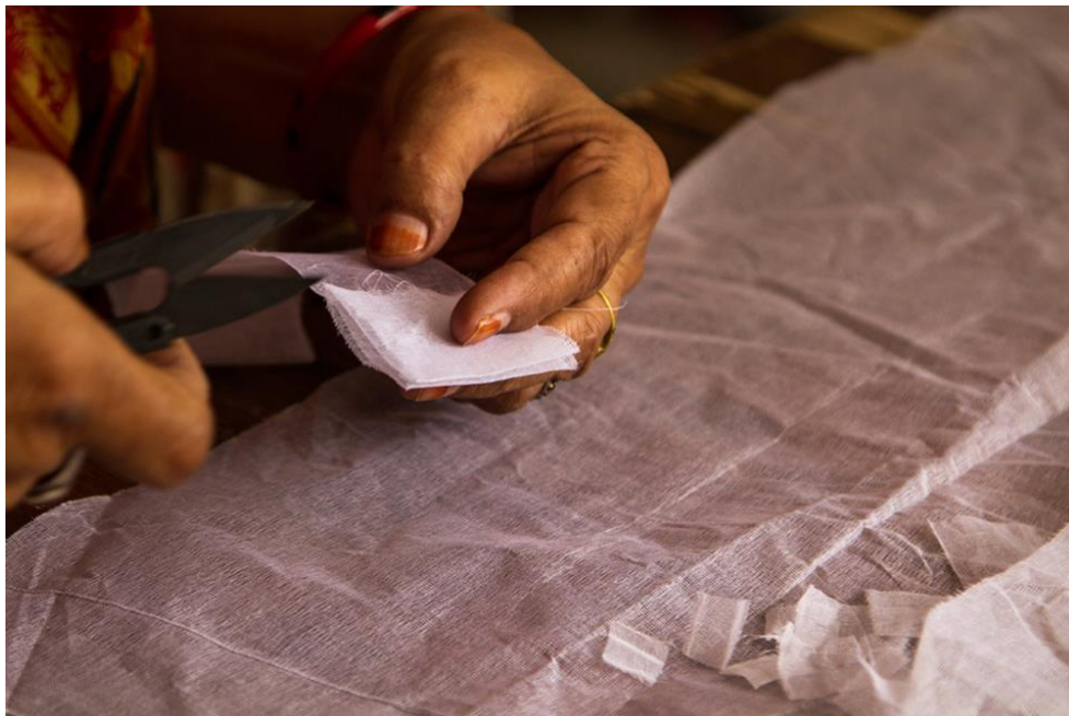
Required color cotton fabric is first cut into equal measurement pieces, Image Source: D'source https://www.dsource.in/gallery/applique-work-aligarh-1#128585
