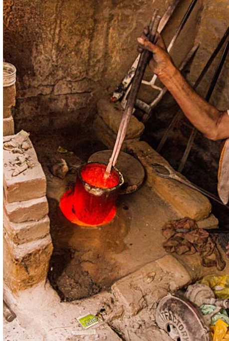
Brass being heated in a furnace, Image Source: D'source https://www.dsource.in/resource/brass-work-aligarh
