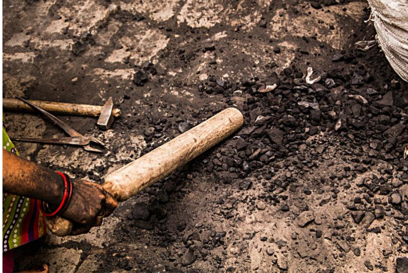
Clay is beaten with wooden mallet to convert them into powder, Image Source: D'source https://www.dsource.in/resource/brass-work-aligarh
