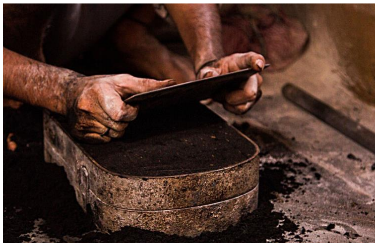
Clay mixture is filled in the frame. Image Source: D'source https://www.dsource.in/resource/brass-work-aligarh
