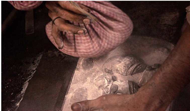
Chalk powder is sprinkled on the mold, Image Source: D'source https://www.dsource.in/resource/brass-work-aligarh
