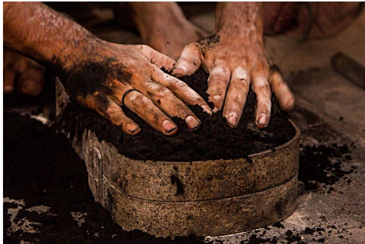
The mixture is filled in the metal frame, Image Source: D'source https://www.dsource.in/resource/brass-work-aligarh
