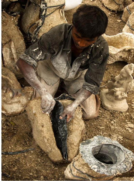
Rubber mould is placed between the Plaster of Paris moulds and then tied together, Image source: D'source https://www.dsource.in/resource/idol-making-aligarh
