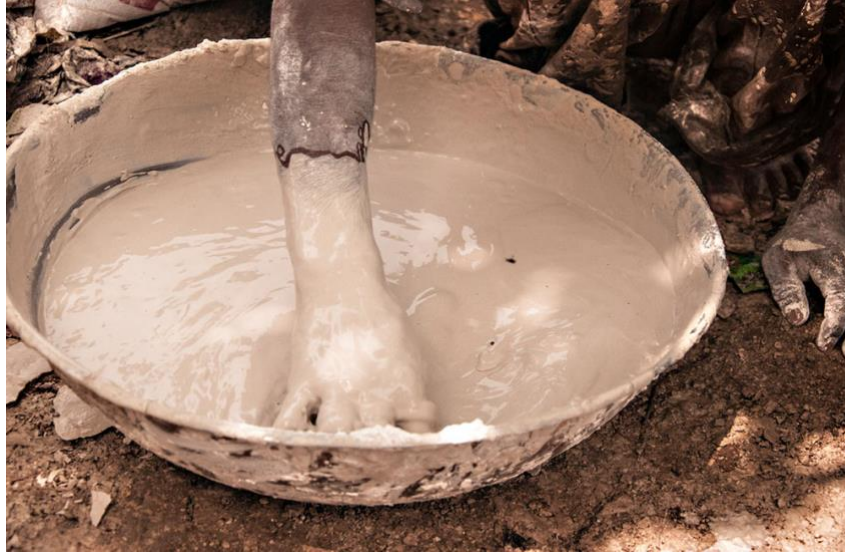
Plaster of Paris solution is first made by mixing it with water, Image Source: D'source https://www.dsource.in/resource/idol-making-aligarh
