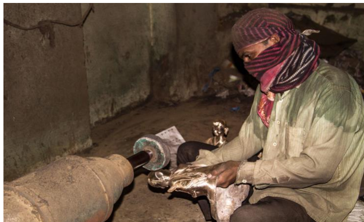
Idols are buffed to smoothen the surface and bring out the shine. Image Source: D'source https://www.dsource.in/resource/brass-work-aligarh
