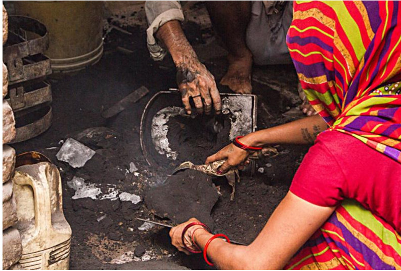
After the moulds are cooled down, the casted metal is scooped out. Image Source: D'source https://www.dsource.in/resource/brass-work-aligarh
