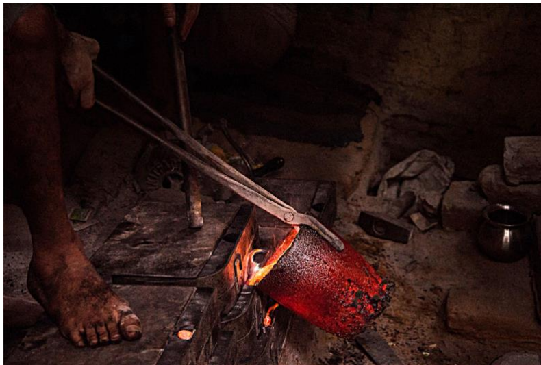
Molten material is poured in the molds. Image Source: D'source https://www.dsource.in/resource/brass-work-aligarh
