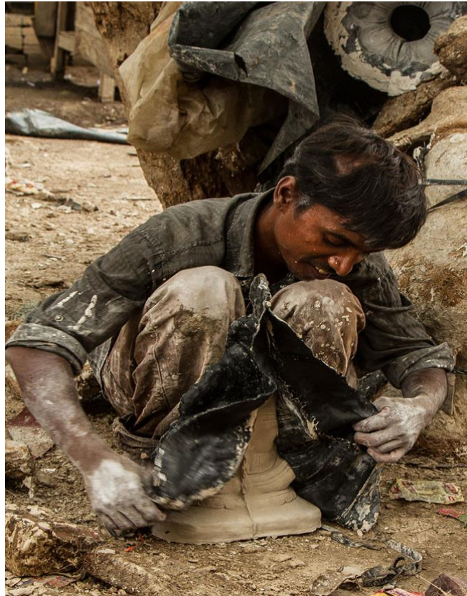
After Plaster of Paris is dried up, it is taken out of the mould, Image source: D'source https://www.dsource.in/resource/idol-making-aligarh
