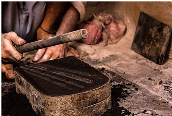
It is beaten it with rod to settle evenly, Image Source: D'source https://www.dsource.in/resource/brass-work-aligarh
