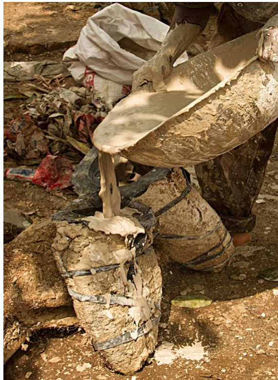
Plaster of Paris solution is then poured into the mold, Image Source: D'source https://www.dsource.in/resource/idol-making-aligarh
