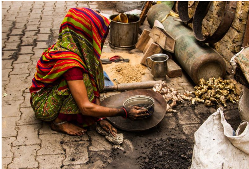
The powder is filtered to get the fine mixture of clay, Image Source: D'source https://www.dsource.in/resource/brass-work-aligarh
