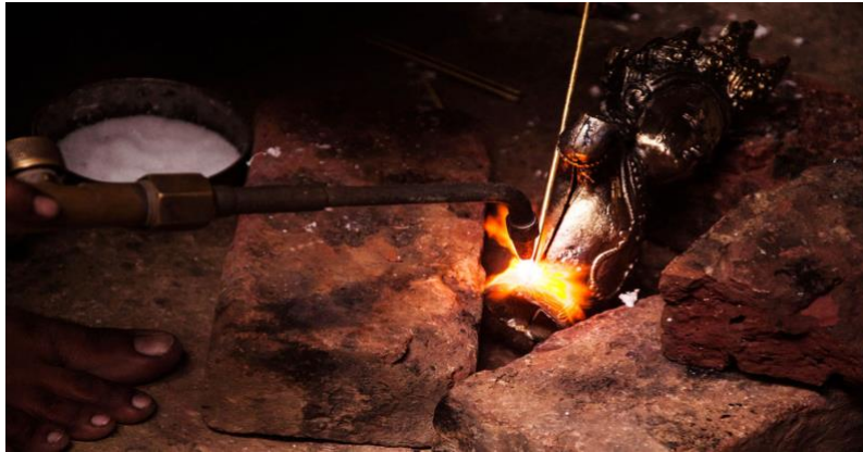
Separate parts of the idol are then soldered together, Image Source: D'source https://www.dsource.in/resource/brass-work-aligarh
