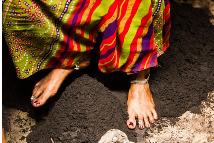
Sand and sugarcane waste is added to clay and mixed well, Image Source: D'source https://www.dsource.in/resource/brass-work-aligarh
