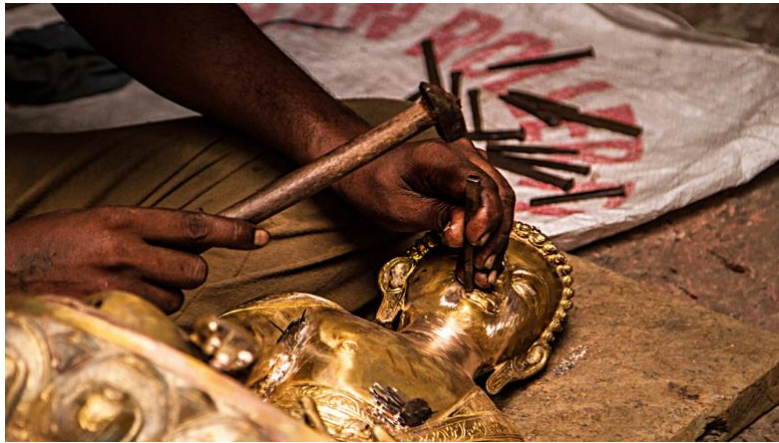
The details are then carved using chisels, Image Source: D'source https://www.dsource.in/resource/brass-work-aligarh
