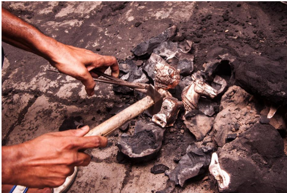
The mould is then broken, and the casted articles are removed, Image Source: D'source https://www.dsource.in/resource/brass-work-aligarh
