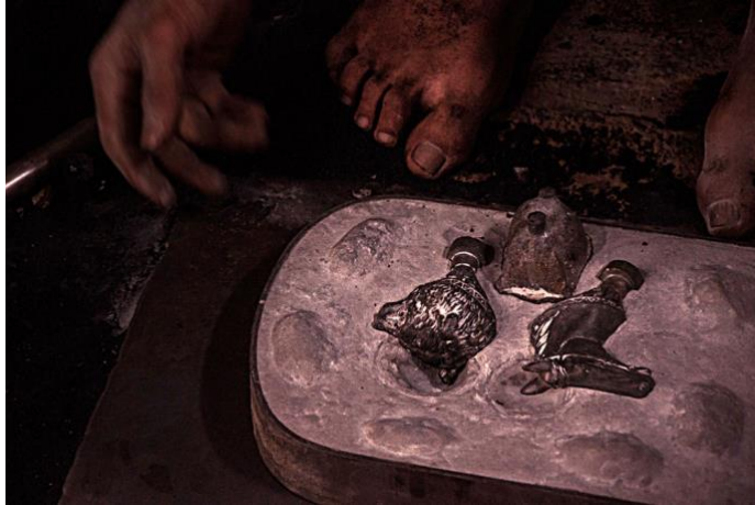
Brass articles are placed so that it leaves the impression on the sand for casting. Image Source: D'source https://www.dsource.in/resource/brass-work-aligarh
